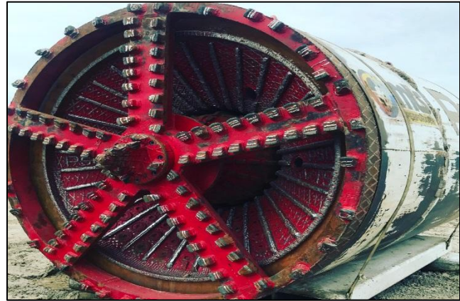
Micro-tunneling boring machine
